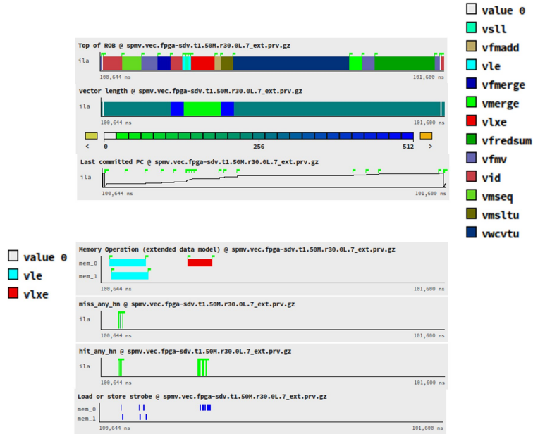
Figure 28: Several timelines for one iteration of the innermost loop of the vector execution. From top to bottom: instruction at the top of the ROB, vector length, program counter, memory operation, L2 misses, L2 hits and data being delivered to the vector unit.
