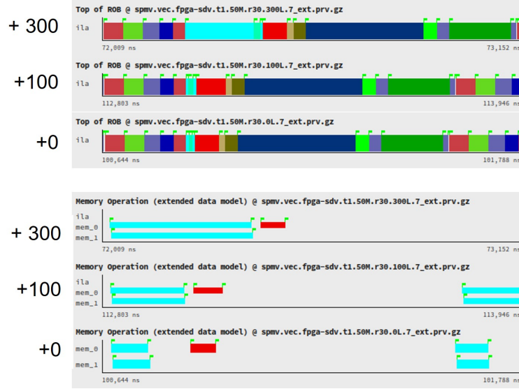
Figure 30: Top of the ROB and memory operations execution timelines for 0, 100 and 300 additional cycles at the memory controller. Only for the 300 cycles case, the additional latency translates into an elongation of the vector load instructions when at the top of the reorder buffer.
