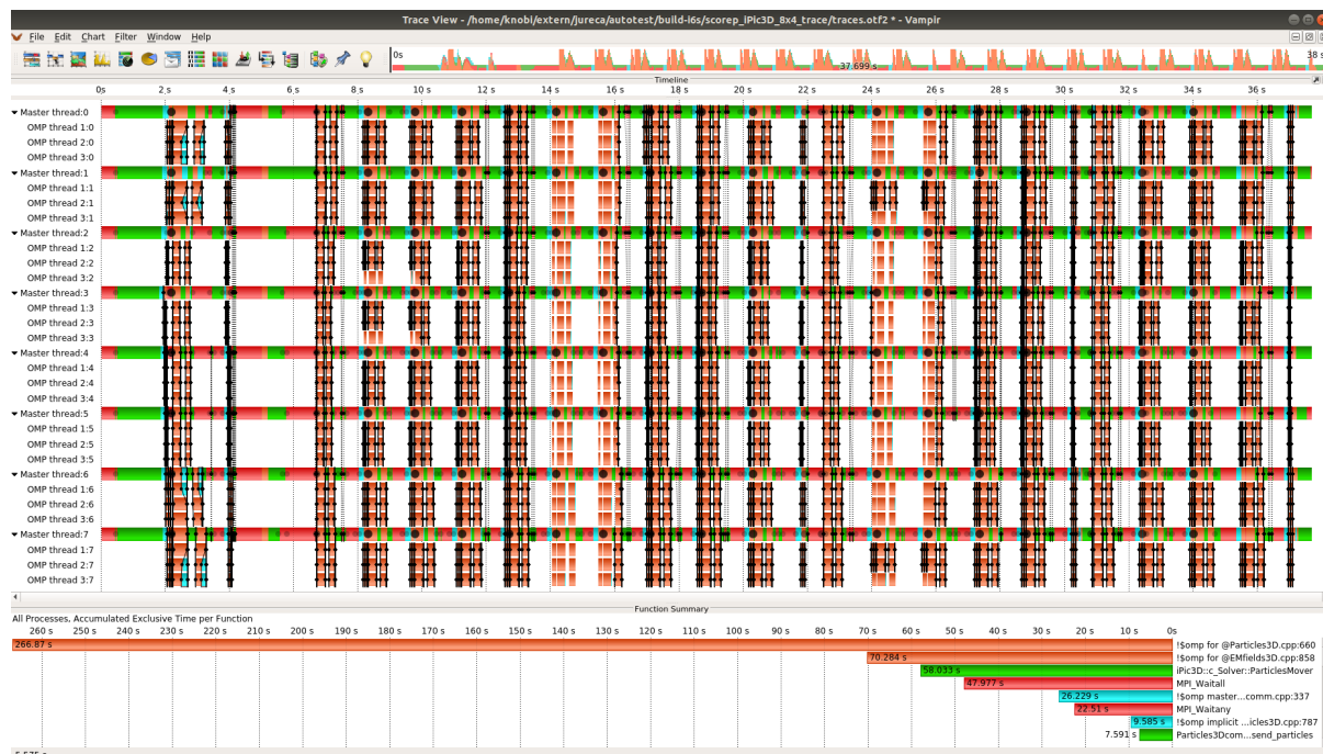
Figure 1: Execution timeline of iPic3D with 20 iterations on JURECA. Timeline chart of the 8 processes at top, and function summary chart at bottom.
